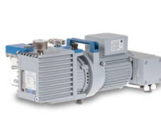
RC 6 Chemistry-HYBRID pump 5.9 m³/h, 2 x 10 -3 mbar Vacuum connection: Small flange DN 16
