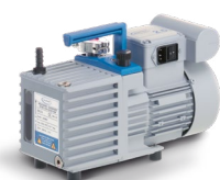
RZ 2.5 Rotary vane pump 2.3 m³/h, 2 x 10 -3 mbar Vacuum connection: Small flange DN 16
