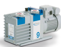
RZ 9 Rotary vane pump 8.9 m³/h, 2 x 10 -3 mbar Vacuum connection: Small flange DN 25
