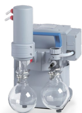
MZ 2C NT +AK +EK Chemistry diaphragm pump 2.0 m 3 /h, 7 mbar Vacuum connection: Hose nozzle DN 8-10
