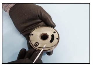
51. Remove the seals on the bearing plate.
