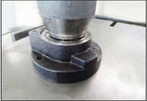
73. Press the shaft seal into the bearing cover as far as it will go.
