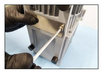
97. Screw the cover of the suction felt.
