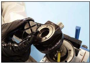
37. Lift the oil pump rotor out of the bearing cover.
