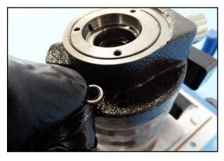
90. Place the Usit rings in the holes of the bearing cover.
