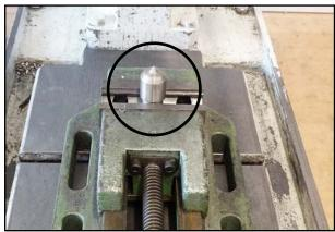
21. Clamp a mandrel, e.g. in a pillar drill or hand lever press.
