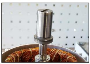
23. Place the coupling on the motor shaft.
