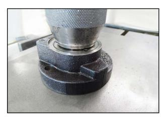
65. Press the shaft seal into the bearing cover as far as it will go.
