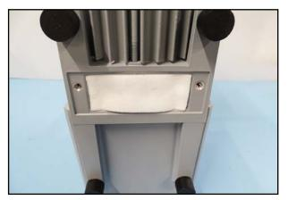
96. Place (new ones if necessary) suction felts in the housing.
