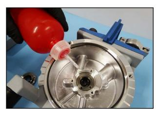
98. Fill the space in front of the removeable sleeve with the vacuum pump oil with which you operate the pump.
