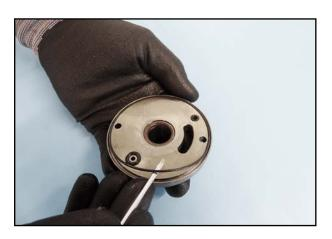
43. Remove the seals on the bearing plate.
