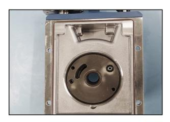
69. Place the bearing plate in the housing.
