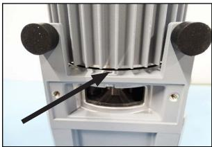
⇒ A gap may occur when inserting the motor.
