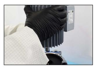
9. Lift the motor out of the housing.
