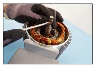
20. Remove the tolerance ring from the motor shaft using a flat blade screwdriver.
