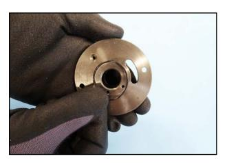
67. Place the O-ring around the bearing plate.
