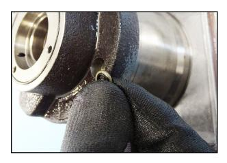
77. Place the Usit rings in the holes of the bearing cover.
