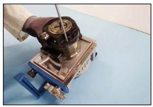
34. Unscrew the screws on the aggregate.
