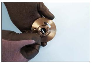
44. Remove the seal on the bearing plate on the other side.
