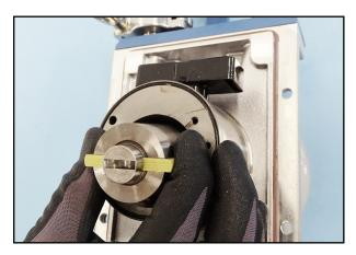
73. Place the rotor with vanes into the stator.
