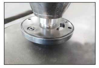
61. Press the shaft seal into the bearing plate as far as it will go.
