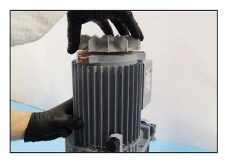
103. Turn the fan wheel slightly until the motor slides completely into the housing.
