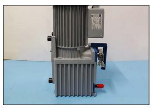
4. Place the pump on the oil reservoir (on the rating plate).
