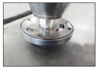
69. Press the shaft seal into the bearing plate as far as it will go.
