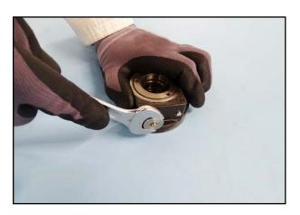
54. Unscrew the screw plug of the oil retention valve from the bearing cover.
