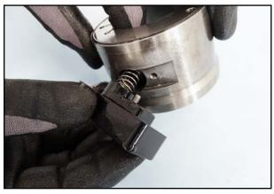
70. Place the oil separator with spring and cap into the stator.
