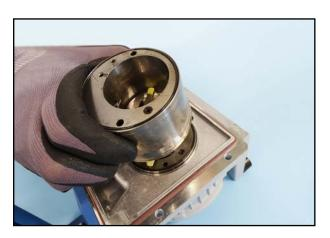
39. Lift off the stator.
