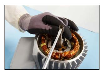
20. Slide a new tolerance ring over the motor shaft using a flat-blade screwdriver.
