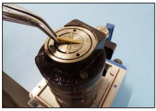
33. Pull the vanes out of the rotor.
