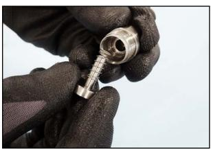
74. Assemble the oil retention valve with housing.
