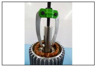
17. Position the puller on the extraction sleeve and coupling as shown.
