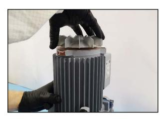
90. Turn the fan wheel slightly until the motor slides completely into the housing.
