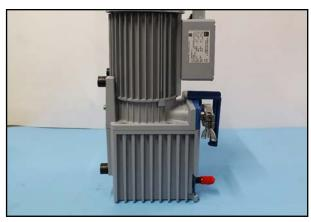
2. Place the pump on the oil reservoir (on the rating plate).
