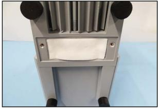
109. Place (new ones if necessary) suction felts in the housing.
