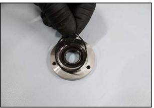
84. Place a new O-ring around the new removeable sleeve.
