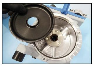
12. Lift the protective wall out of the housing.
