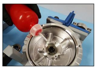
16. Fill the space in front of the removeable sleeve with the vacuum pump oil with which you operate the pump.
