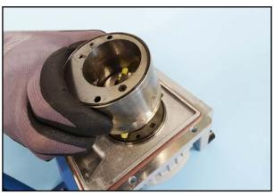
47. Remove the stator.
