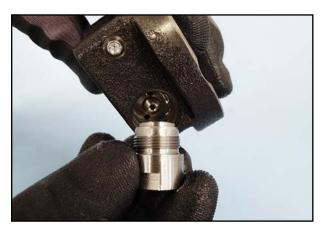
75. Screw the retaining device into the bearing cover.
