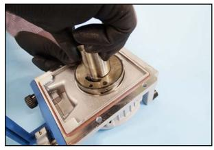
49. Lift off the rotor and the bearing plate.
