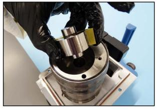
85. Place the rotor with vanes into the stator.
