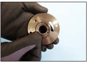
75. Place the O-ring around the bearing plate.
