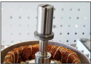
24. Place the coupling on the motor shaft.
