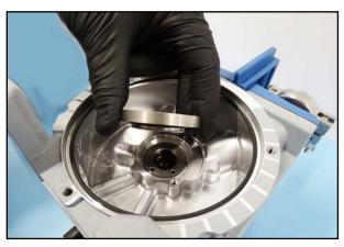
28. Lift out the removeable sleeve.
