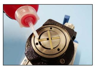
94. Fill the space around the rotor with the vacuum pump oil with which you operate the pump.
