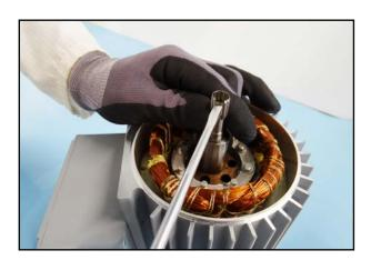
21. Slide a new tolerance ring over the motor shaft using a flat-blade screwdriver.
