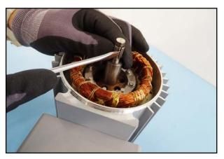
19. Remove the tolerance ring from the motor shaft using a flat blade screwdriver.
