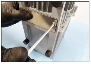
110. Screw the cover of the suction felt.
