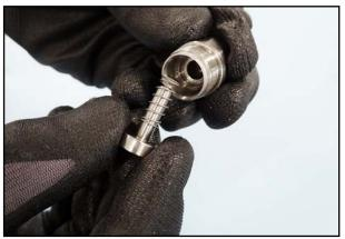
87. Assemble the oil retention valve with housing.
