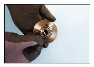
52. Remove the seal on the bearing plate on the other side.
