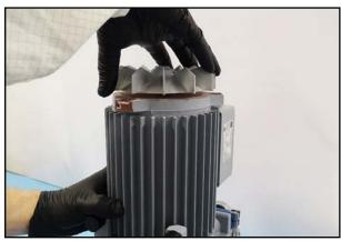
21. Turn the fan wheel slightly until the motor slides completely into the housing.
