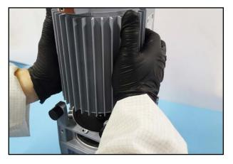
102. Carefully place the motor in the housing.
