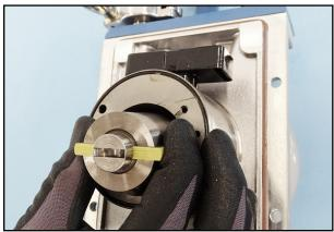
81. Place the rotor with vanes into the stator.
