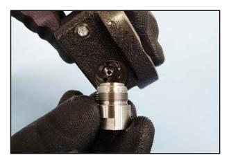
88. Screw the retaining device into the bearing cover.
