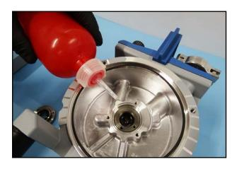
85. Fill the space in front of the removeable sleeve with the vacuum pump oil with which you operate the pump.
