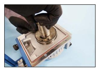
41. Lift off the rotor and the bearing plate.
