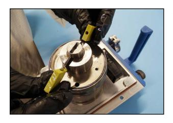
40. Pull the vanes out of the rotor.
