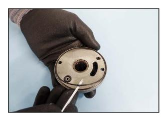
76. Place the O-rings in the bearing plate on the opposite side.
