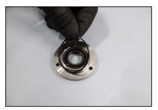
15. Place a new O-ring around the new removeable sleeve.
