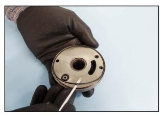
68. Place the O-rings in the bearing plate on the opposite side.
