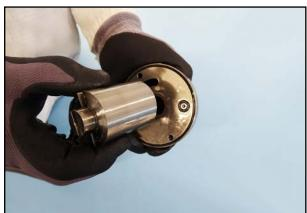
42. Pull the rotor and the bearing plate apart.
