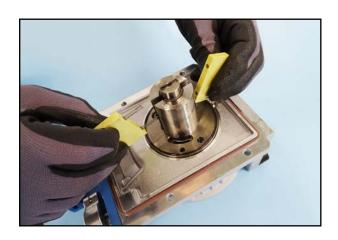
48. Pull the vanes out of the rotor.
