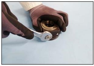
46. Unscrew the screw plug of the oil retention valve from the bearing cover.
