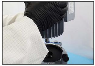
11. Lift the motor out of the housing.
