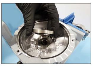
27. Lift out the removeable sleeve.
