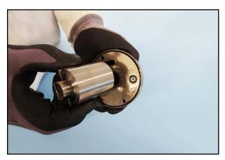
50. Pull the rotor and the bearing plate apart.
