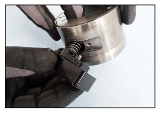
78. Place the oil separator with spring and cap into the stator.
