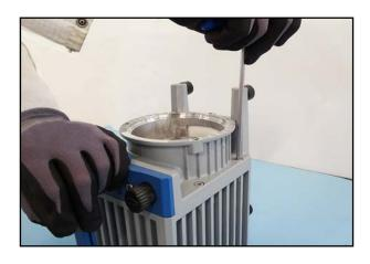
96. Screw the aggregate to the oil reservoir.
