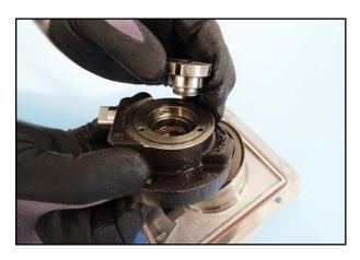
37. Lift the oil pump rotor out of the bearing cover.
