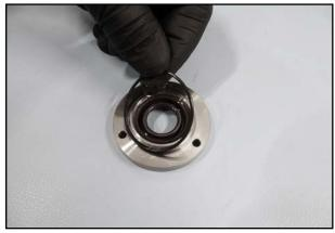
97. Place a new O-ring around the removeable sleeve.
