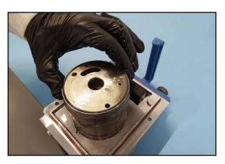
82. Insert the intermediate bearing plate.
