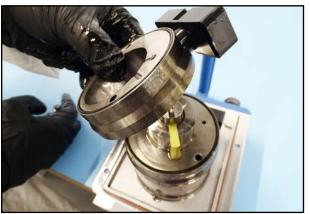
39. Lift off the stator.
