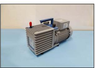
111. Place the pump on the pump feet.
