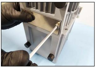
28. Screw the cover of the suction felt.
